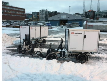
Figure 4 Paxster electric quadricycle (left) and Velove cargo cycles (right) are two examples of LEFVs. Photo credit: Howard Weir
