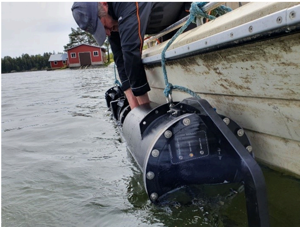
Figure 5 appendix Battery change in the autonomously moving deterrent. Photo: E. Lehtonen
