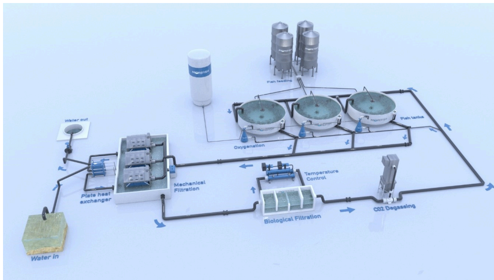
Figure 1. Schematic of a recirculating aquaculture system
