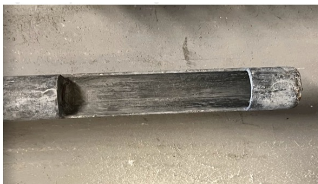
Figure 3.28. Typical sampling hole (A) and sampling rod (B). Photo: Kredsløb.
