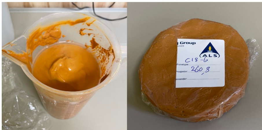
Figure 3.14. Sludge before and after dewatering in a Folldal lab test. Photo: DMF.
