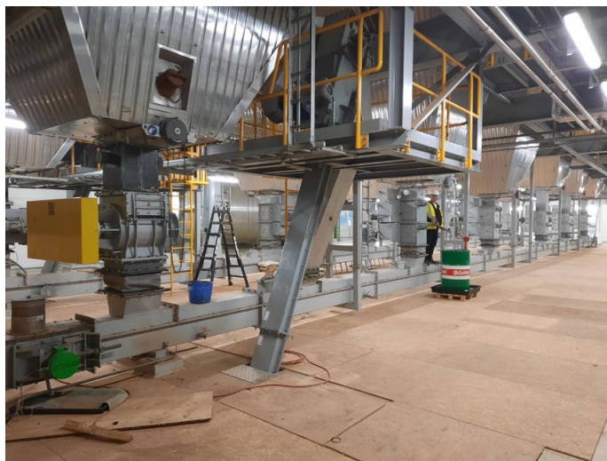
Figure 3.29. Sampling hole and sampling rod at ARGO's MSWI facility (A). A view of several FA precipitation stages connected to a conveyor belt line on the bottom (B). All stages were sampled during the project. Photos: ARGO.
