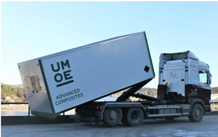
Figure 4. Hook-loaded hydrogen transport and storage module by UAC (UAC, 2018).
