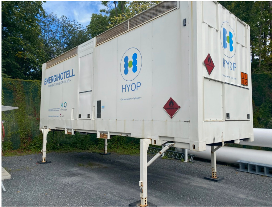
Figure 3. The Energy Hotel hydrogen transport and storage solution. The Energy Hotel technology is the IPR of Hynion AS. Source: Hynion AS.
