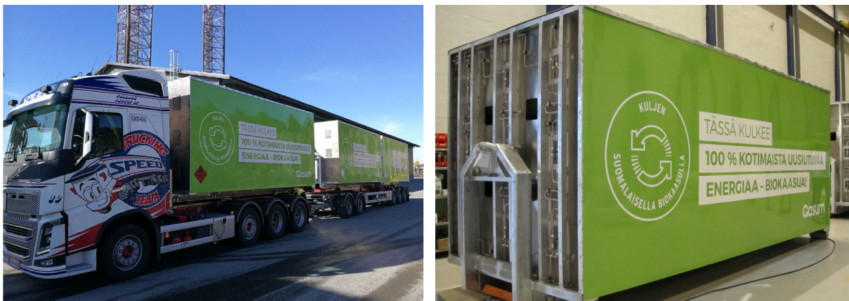
Figure 2. On left: Gasum biogas transport by Speed Group Oy. On right: 20 ft container used by Gasum 15 .
