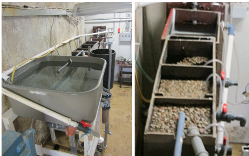
Figure 2.1-4: Overview of the fish tank, swirl separator, and pumice biofilter. Photo: Matorka
